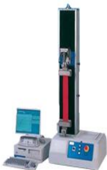
2.16-rasm.UM-Lab3 asbobi tolalarning cho‘zilishdagi mustahkamligini aniqlash.
