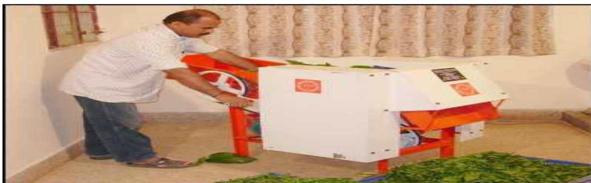
22-rasm. Avtomatik barg to'g'ragich asbobi 2
