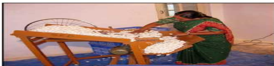
26-rasm. Pillalarni losdan tozalaydigan dastgoh.
