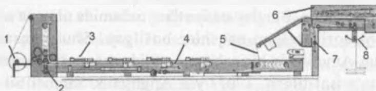
209- rasm. Yassi andozali gul bosish mashinasining sxemasi:
