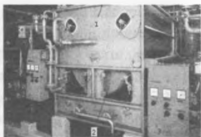
74- rasm. "Trikofleks – 2000" yuvish mashinasining tashqi ko'rinishi:
