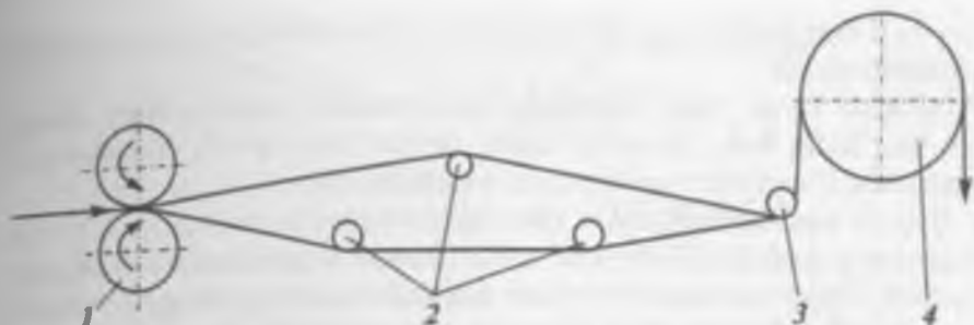
56-rasm. Iplarni nam holda ajratishning prinsipial chizmasi.
