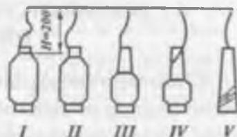
3-rasm. Tuftakdan ipni o'rash jarayonida taranglikning o'zgarishi.
