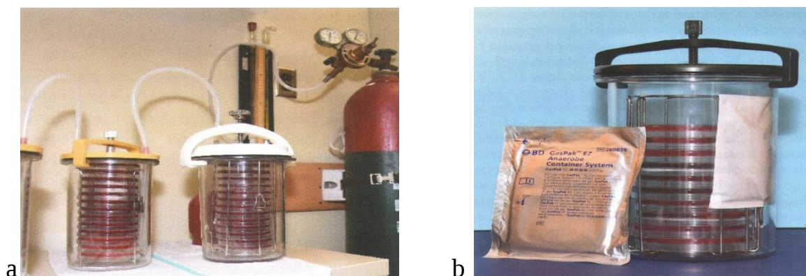
44-rasm. Anaerostatlarda kimyoviy usulda anaerob sharoit yaratish.
