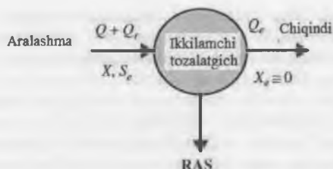
64-rasm. Ikkilamchi tindirgich atrofidagi qattiq muallaq zarrachalar uchun moddiy balans.
