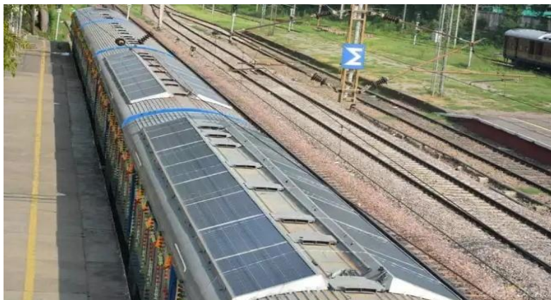
25-rasm. DEMU (Diesel Electric Multiple Unit) quyosh panellari bilan jihozlangan ilk poezd (Hindiston).
