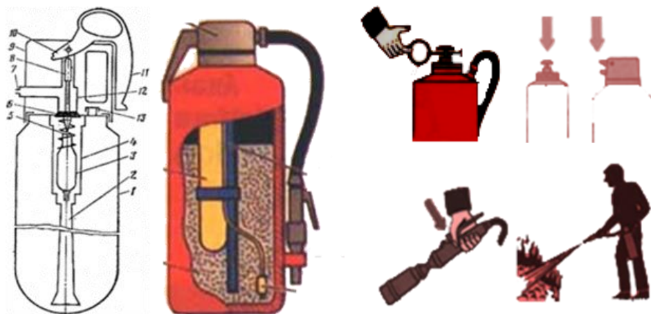
10.1-rasm. OP-1 turdagi o't o'chirgich tuzilishi va undan foydalanish 1- korpus; 2 -sifonli quvurcha; 3- ishchi gazi uchun ballon; 4- gaz ballon uchun stakan korpusi; 5-membrana; 6- klapan; 7- sepgich tirqishi; 8-shtok; 9- kallak qalpog'i; 10 -xvostovik ; 11- dastak; 12 - kallak; 13-tiqin.
