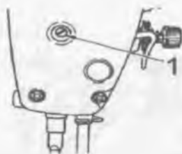
21-rasm Tepkini holatini sozlash
