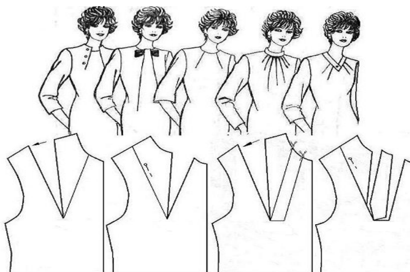
17-rasm. Ko'krak vitochkasini old bo'lak bo'yin o'mizi chizig'iga ko'chirish
