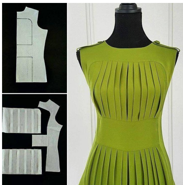
26-rasm. Ayollar ko'ylagining old detalini parallel kengaytirish va taxlamalar modellashtirish
