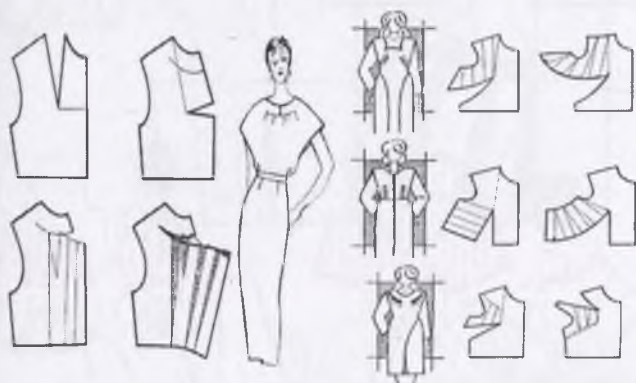
41-rasm. Ayollar kiyimida murakkab burmalar, qirqimlar va drapirovkalar modellashirish
