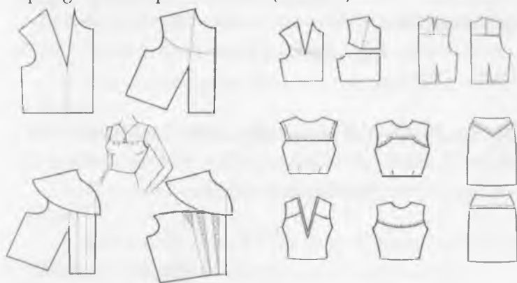
19-rasm. Yelkaga oid va belga oid ayollar kiyimida gorizontallik bo'laklash usulini qo'llab koketkalar modellash
