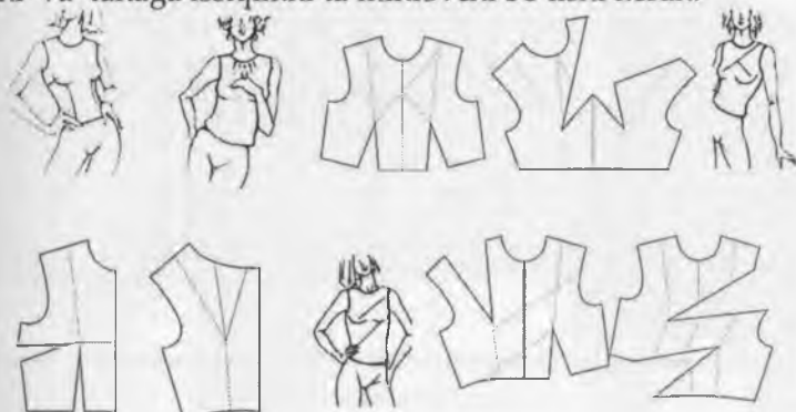
155-rasm. Trikotajdan ayollar ko'ylagini modellashirish: vitochkalarni oddiy ko'chirish
