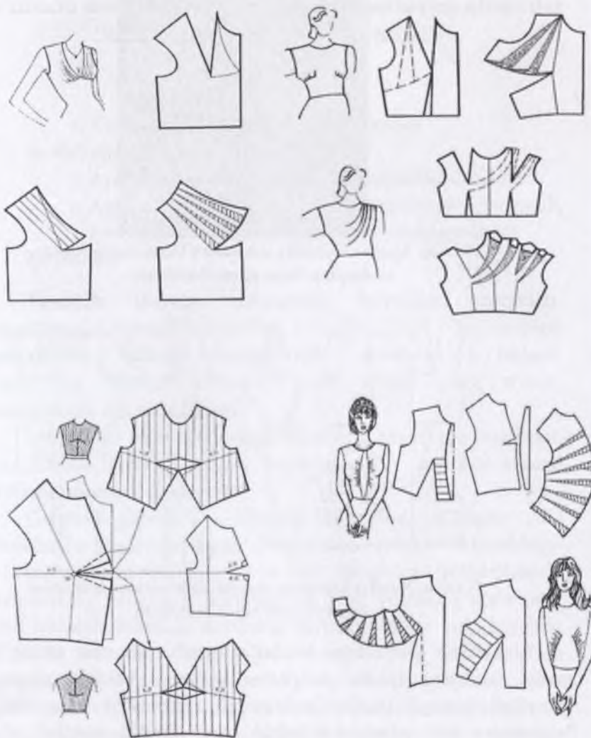
42-rasm. Ayollar kiyimida murakkab burmalar, qirqimlar va drapirovkalar modellashirish
