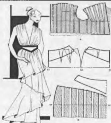
156-rasm. Trikotajdan ayollar ko'ylagini modellashtirish: detallarni parallel kengaytirish
