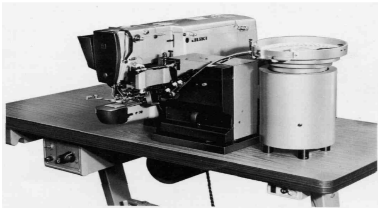
98-rasm. LK-981-555/BR-2 tugma qadash yarim avtomatining tashqi ko'rinishi.
