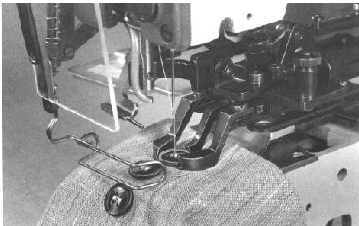
97-rasm. b. Tugma qadalish jarayoni.
