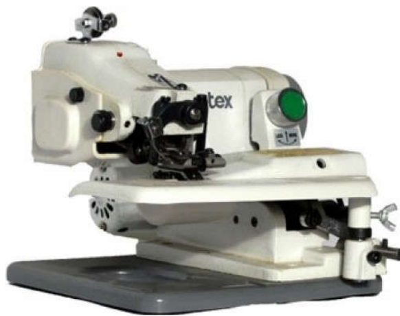
27-rasm. Protex firmasining TY-600 markali bir ipli yashirin baxyaqator tikish mashinasi
