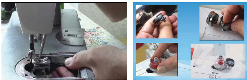
Figure 3.4. The work to be done during the automatic filling of the shuttle tube
