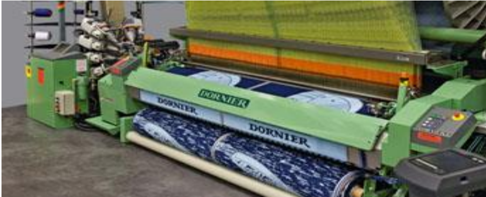
Air-jet Terry weaving machine ServoTerry®
