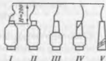
3-rasm. Tuftakdan ipni o'rash jarayonida taranglikning o'zgarishi.
