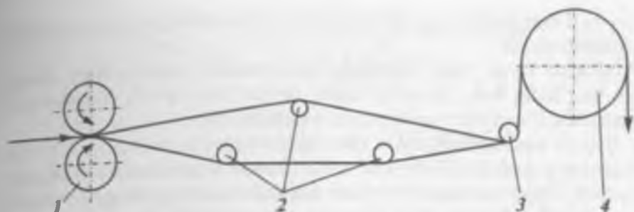
56-rasm. Iplarni nam holda ajratishning prinsipial chizmasi.
