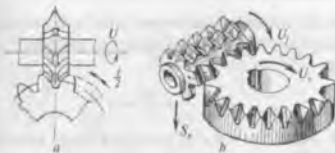
34-rasm. Nusxa ko'chirish usulida modulli disk frezalar (a) va chervyak modulli frezalar (b) bilan tishli g'ildirak tishlarini ishlash.
