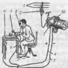
4-rasm. Dastaki payvandlash posti: 1 – tok tarmog'i; 2 – ulagich; 3 – tok o'zgartirgich; 5-6 – elektr simi; 6 – zagotovka; 7 – elektrod turkichi; 8 – shit; 9 – stol; 10 – tok rostlagich.
