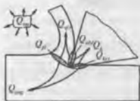
47-rasm. Qirg'ish jarayonida issiqlik manbalari va uning bo'linishi (taqsimlanishi).
