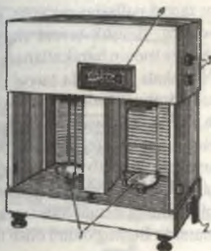
9.2-rasm. Ikki pallali VLR-200 rusumli analitik tarozi: 1-pallalar; 2-arretir; 3-milligramm massali toshchalarni o'rnatish dastalari; 4-o'lchash natijasini yozib olish ekrani
