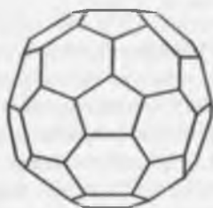
Fig. 4.6 Structure of C_{60} .
