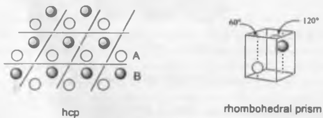
Fig. 2.5 Different expressions of hexagonally close-packed.
