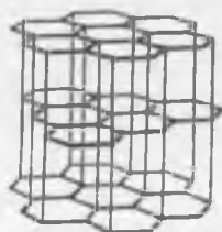
Fig. 4.4 Structure of graphite.
