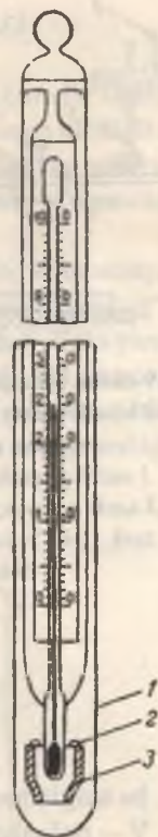
18-rasm. Tomchilash temperaturasini aniqlash asbobi: 1-probirka; 2-gilza; 3-idishcha
