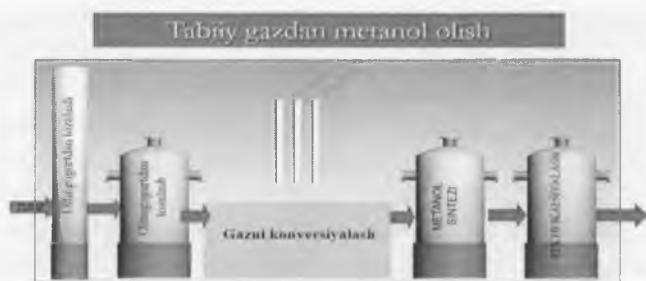
16.3-rasm. Metanol olishning soddalashtirilgan sxemasi:
