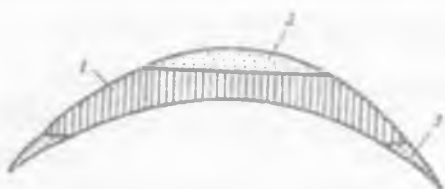
V.14-rasm. Ikkilamchi gaz qalpoqli neft konining sxemasi: 1-neft, 2-gaz qalpog'i; 3-chegara tashqarisidagi suv
