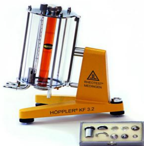
82 – rasm. KF 3.2 modeli harakatlanuvchi sharchaliu Geppler viskozimetri
