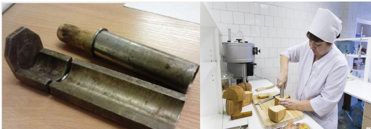
10-rasm. Nonning g‘ovakligi Juravlyova asbobi yordamida aniqlanishi.
