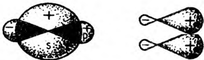
1.3-Rasm. Uglerodning s va p orbitallaring gibridlanishi
