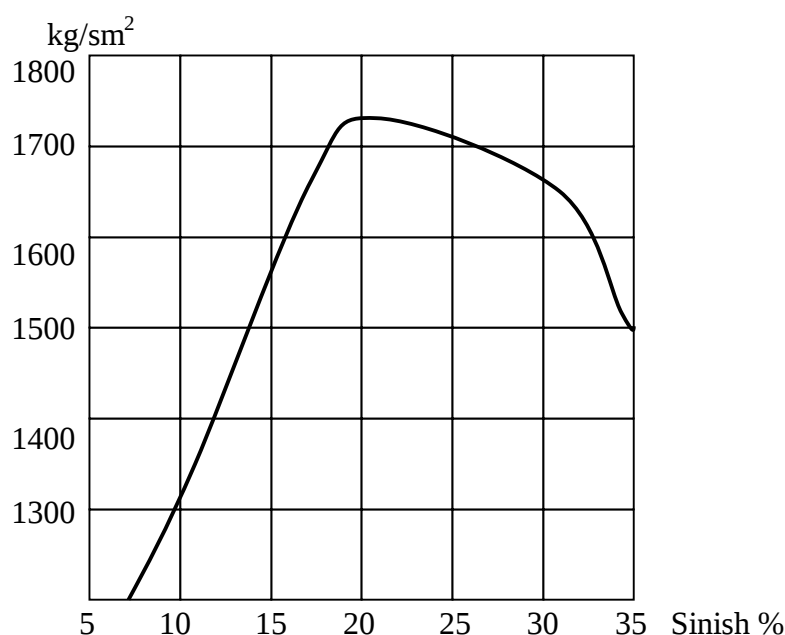
3.4-rasm. Toshko'mir smolasining uglerod-grafit materialning cho'zilishdagi mustahkamligiga ta'siri.
