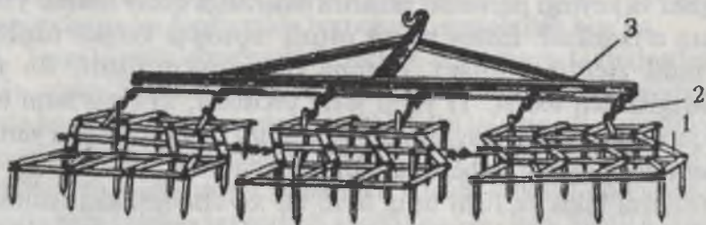
13-rasm. Tishli borona. 1-zveno; 2-pishang; 3-zanjir.
