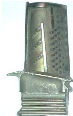
10.3-rasm. Gaz trubinasi lopatkasining ichki tuzilishi
