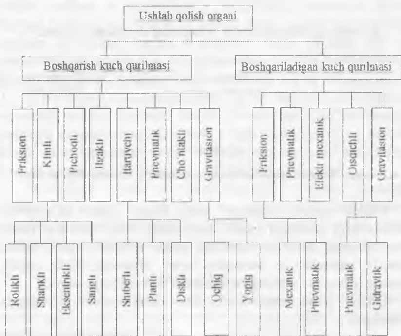
4.3-rasm. Ushlab qolish organlarining tasnifi
