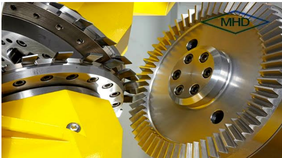
9.7 – rasm. Keskichli tish qirqish kallagida konusli tish qirqish jarayoni.
