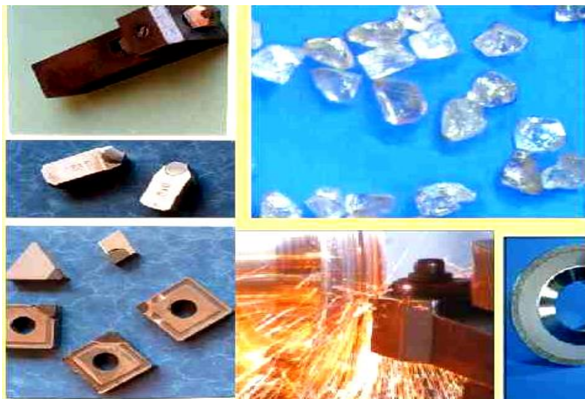
1.7 - rasm. Kesish asboblari uchun kubsimon BOR nitridli o'ta qattiq materiallar.
