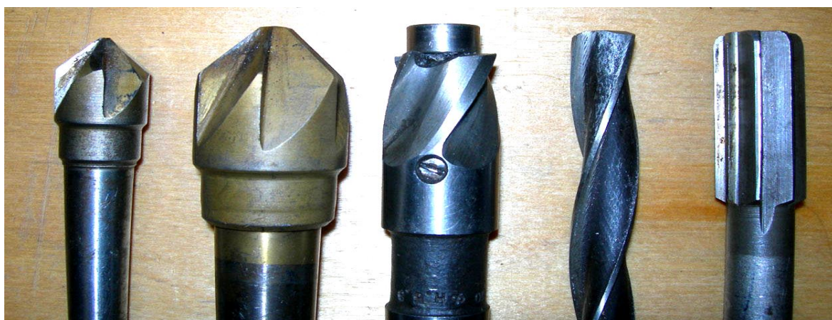
3.13-rasm. a - Zenkovka, b –sozlanadigan zenker, c – zenker, d – razvyortka.
