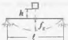
11.10 – rasm. Zarb ta'sirida egilish
