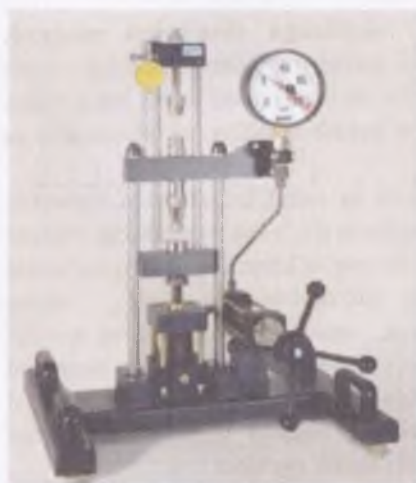
2.15 – rasm [33]. 1-dinamometr; 2-qamrab ushlovchi; 3-yuqori plita; 4-doiraviy shkalalik o'lchov asbobi; 5-namuna (transportlovchi fiksator); 6-yo'naltiruvchi rama; 7-bosh tsilindr bilan maxovik; 8-pastki plita; 9- bosh tsilindr; 10-tayanch pyatasi; 11-transportlash rukoyatkasi
