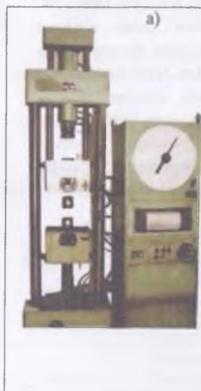
2.15 – rasm [33]. 1-dinamometr; 2-qamrab ushlovchi; 3-yuqori plita; 4-doiraviy shkalalik o'lchov asbobi; 5-namuna (transportlovchi fiksator); 6-yo'naltiruvchi rama; 7-bosh tsilindr bilan maxovik; 8-pastki plita; 9- bosh tsilindr; 10-tayanch pyatasi; 11-transportlash rukoyatkasi
