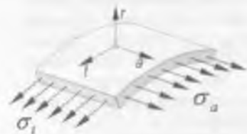
3.40-rasm. Devorlardagi tekis kuchlanish holati
