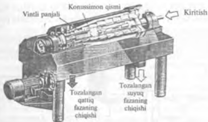
23.5-rasm. WESTFALLA SEPARATOR firmasining shlamga ishlov berish uchun dekantator moslamasi.
